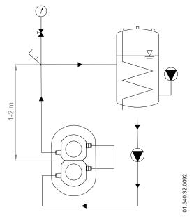
Auxiliary fluid pipes are recommended to be made of stainless steel and as short and straight as possible so the auxiliary fluid can flow easily.
