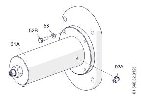
4. Separate the cover and the bypass casing (01A) from each other until a 17 mm open-end spanner can be used to unscrew the cover + piston assembly from the rest of the bypass.
