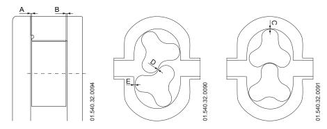
The following table details the distances required for synchronising and adjusting the rotors. The included distances are:
