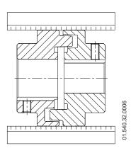
check the maximum alignment deviations shown in the figure do not exceed those indicated in the table below:
