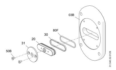
12. Place the bypass casing (01A) in the pump cover (03B) and screw the piston (20) to the inner piston (20A) using a 17 mm open-end spanner.
