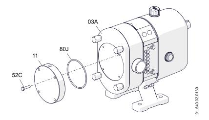
To fit the front heating chamber to the pump, the O-ring (80J) needs to be placed on the back cover (11) and secured to the cover (03A) using the screws (52C).
